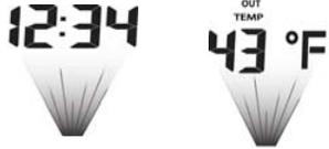
**IMPORTANT:** When operating on a/c power, to avoid interference, the projection will turn off while the Projection Alarm searches for the WWVB signal. The projection will return after the 2-10 minute search which occurs during the late night or early morning hours.
